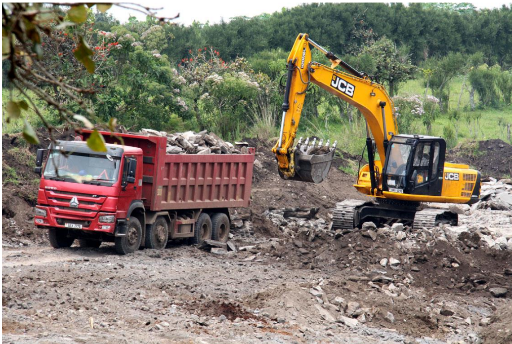
Picture 2: An excavator loads pozzolana on a large truck in a mechanised mine. © TLC
